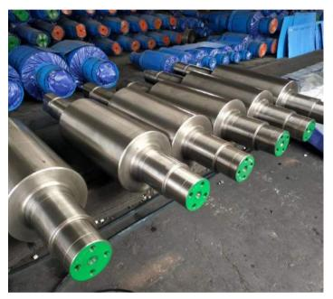
**Sleeves** by centrifugal casting and shaft of forged steel, applicable to various sections and rail & beam mills. Material covers SGP, SGA, Adamite and K Metal, GT Adamite.
