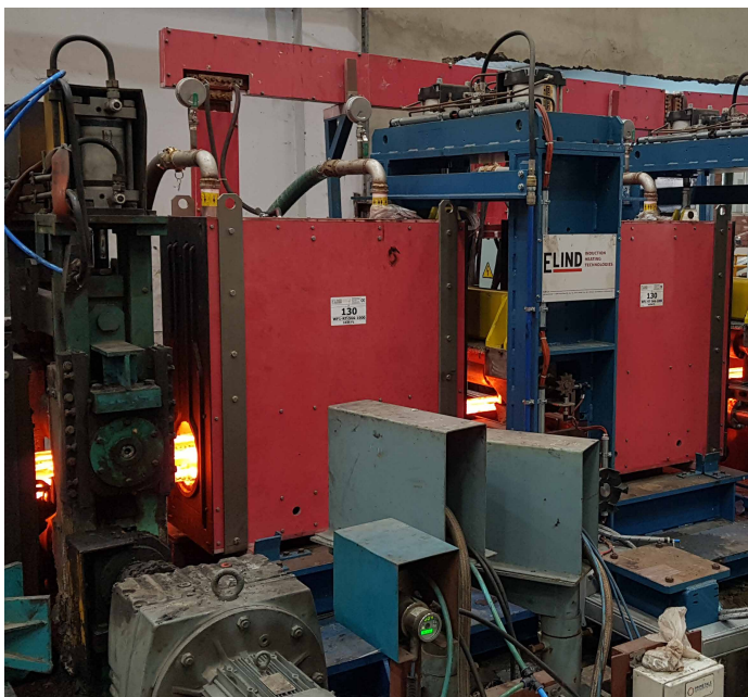
Billet Induction Heater Execution of Commissioning at Naveena Steel
